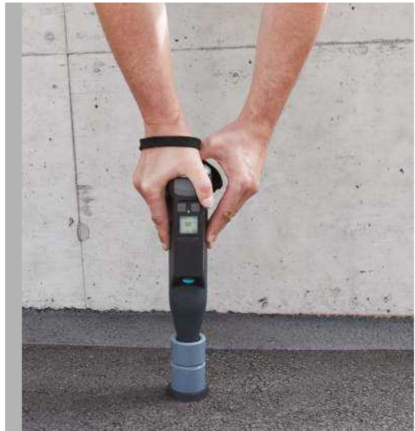
Original Schmidt Live with portable testing anvil
