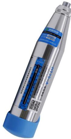
Used for testing the compressive strength of ordinary concrete in the range of 6 ~ 30Mpa in structural engineering
